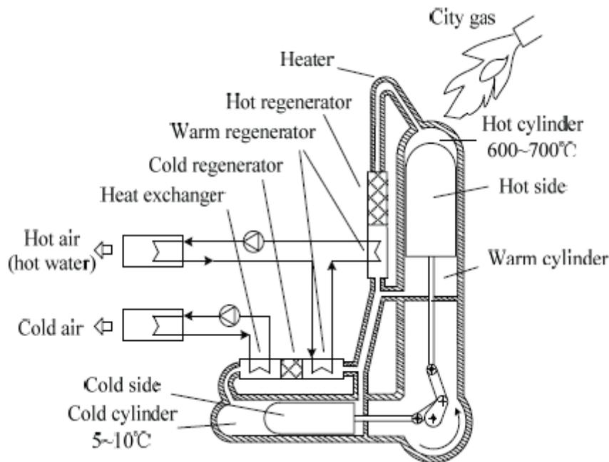
**Figure C-21: Schematic of kinematic Vuilleumier heat pump**
